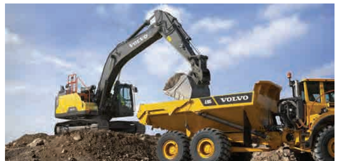
BOTTOM: Volvo's novel hydraulic hybrid harvests 'free' energy generated by the down motion of the excavator's boom.
