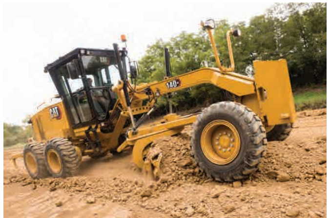
LEFT AND FAR LEFT: The Cat C7.1 engine, 6F/3R automatic powershift transmission (that eliminates the inching pedal), and precisely designed hydraulic system ensure the balanced performance of the machine in all operating situations.
