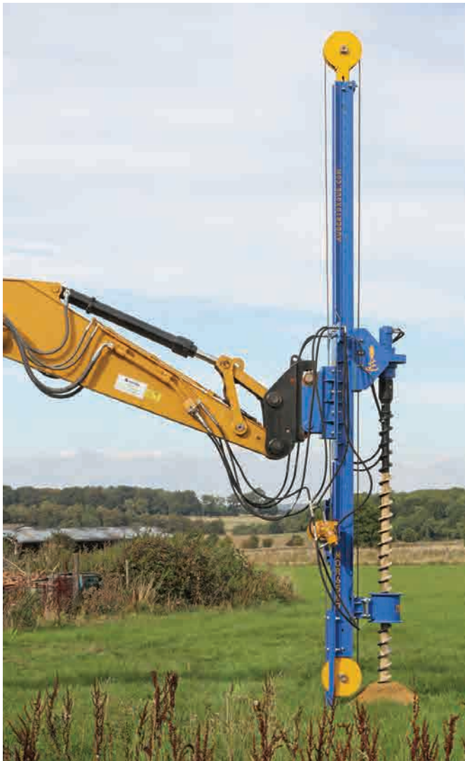
ABOVE AND LEFT: The mast-based drilling rig from Auger Torque is designed for accurate, quick and efficient drilling of large quantities of equal diameter holes. It is suitable for use with excavators between 12 and 15 t, with a torque range from 2,717 to 8,152 Nm.
