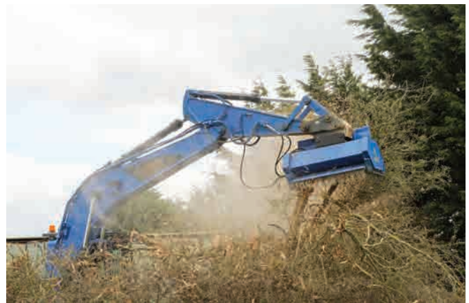
The multipurpose mulcher attachment can be used with 5- to 15-t excavators as well as skid steer loaders.
