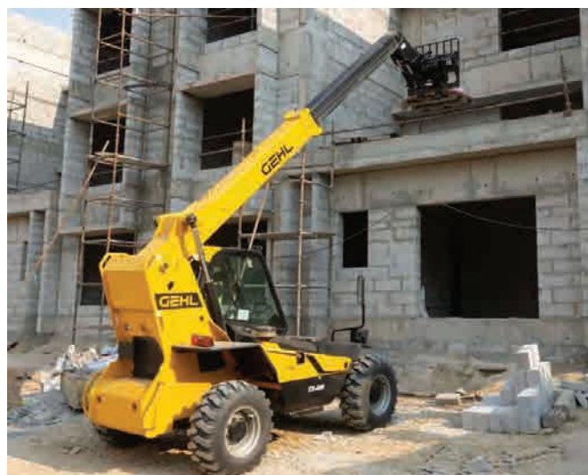
TOP AND ABOVE: Manitou MXT 840 and Gehl TX 408 telehandlers provide a 7.60 m lifting height for a maximum capacity of 4 t.
